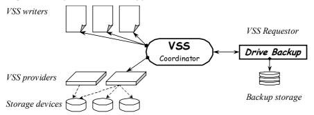
VSS itself only coordinates activity of providers, writers and requestors. A standard Windows XP/2003 distribution includes the VSS coordinator, the universal software provider (VOLSNAP), several VSS writers for system components and the universal VSS writer for MS Desktop Engine (MSDEwriter). In the near future there is hope of an Oracle VSS writer.
