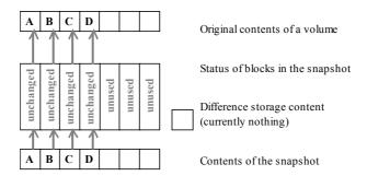
2. Some application tried to modify the block B. Before modifications are made, the snapshot provider copies contents of the block B to the difference storage. The block is now marked as "changed". Then the block B is updated. The snapshot will redirect all queries to the block B to data stored in the difference storage. Queries to blocks A, C and D will be directed to appropriate blocks of the volume.
